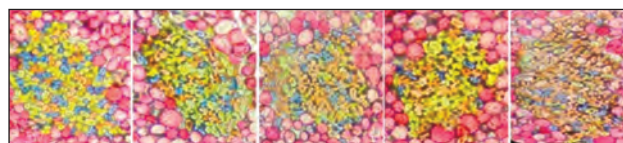
Fig. 5. Three-component yarn blended by one passage of drawing: a – (14–18); b – (19–23)
