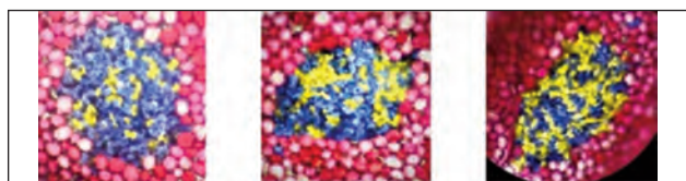
Fig. 3. Two-component yarn blended by three passage of drawing (6–7)
